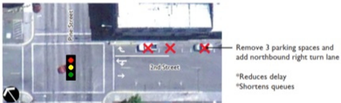
Figure 16: New 2 nd Street lane configuration
