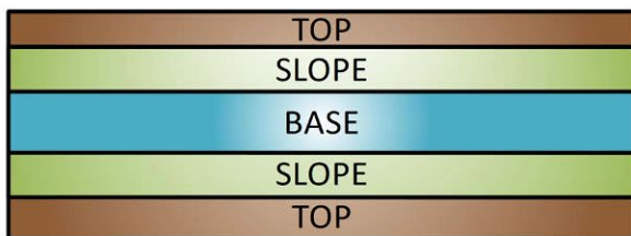
Figure A-1. Wetland status indicator for the moisture zones found in a vegetated stormwater BMP.
