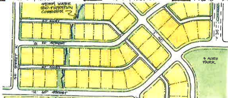
SINGLE FAMILY DETACHED HOMES 230 UNITS 1" = 100'-0", 46.5 AC. TO 10,000 SF LOTS NOTE: ALL ACREAGES INCLUDE STREETS, PARKS & DRAINAGE WAYS
