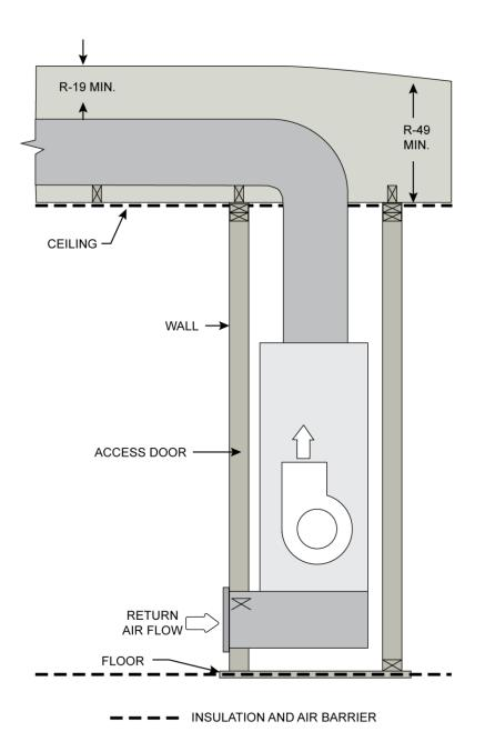
Figure 2: Air handler in crawl space or garage
