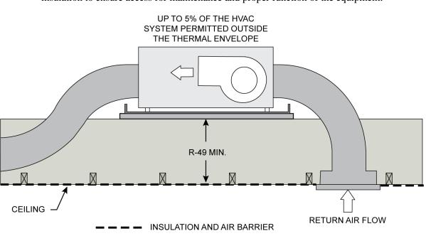
**Figure 3:** Air handler in attic, with 5% allowance. The unit shall not be buried in insulation to ensure access for maintenance and proper function of the equipment.
